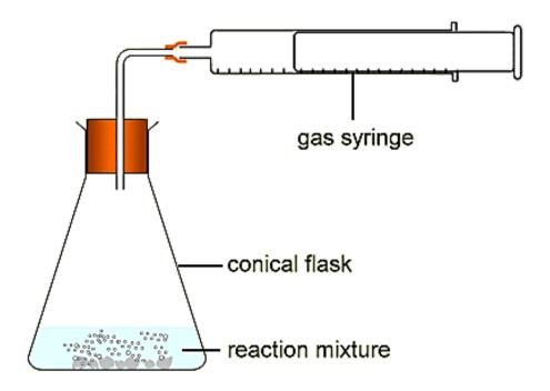
Some students carried out an investigation into the effect of concentration of nitric acid on the rate of this reaction, by combining 20.0 mL of dilute nitric acid of various concentrations, with 0.10 g of magnesium ribbon.
